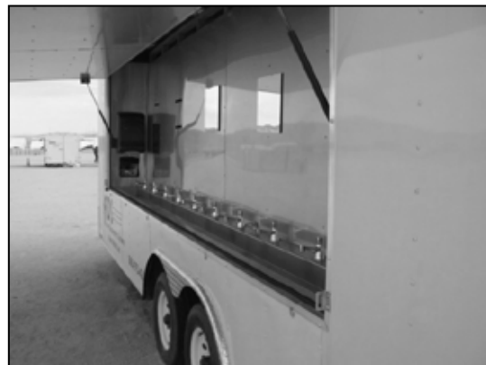
Figure 44. Typical open air wash stations with push-button fixtures.
